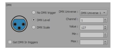
Now Art-Net IN allow DMX signal to trig the software and the software play Art-Net to the nodes configured as output.
